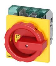
SENTRON, Molded case switch 3LD5 UL, Emergency switching-off, 4-pole, certified according to UL489 UL60947-4-1 and IEC60947-3, UL: 30A, SCCR 50kA at 480VAC, Operating power at 480VAC 3-phase: 20hp, IEC: 32A, Operating power at AC-23A at 400V: 15kW, front-mounted, rotary operating mechanism, red/yellow, 4-hole mounting of the handle, incl. terminal covers for the infeed side
