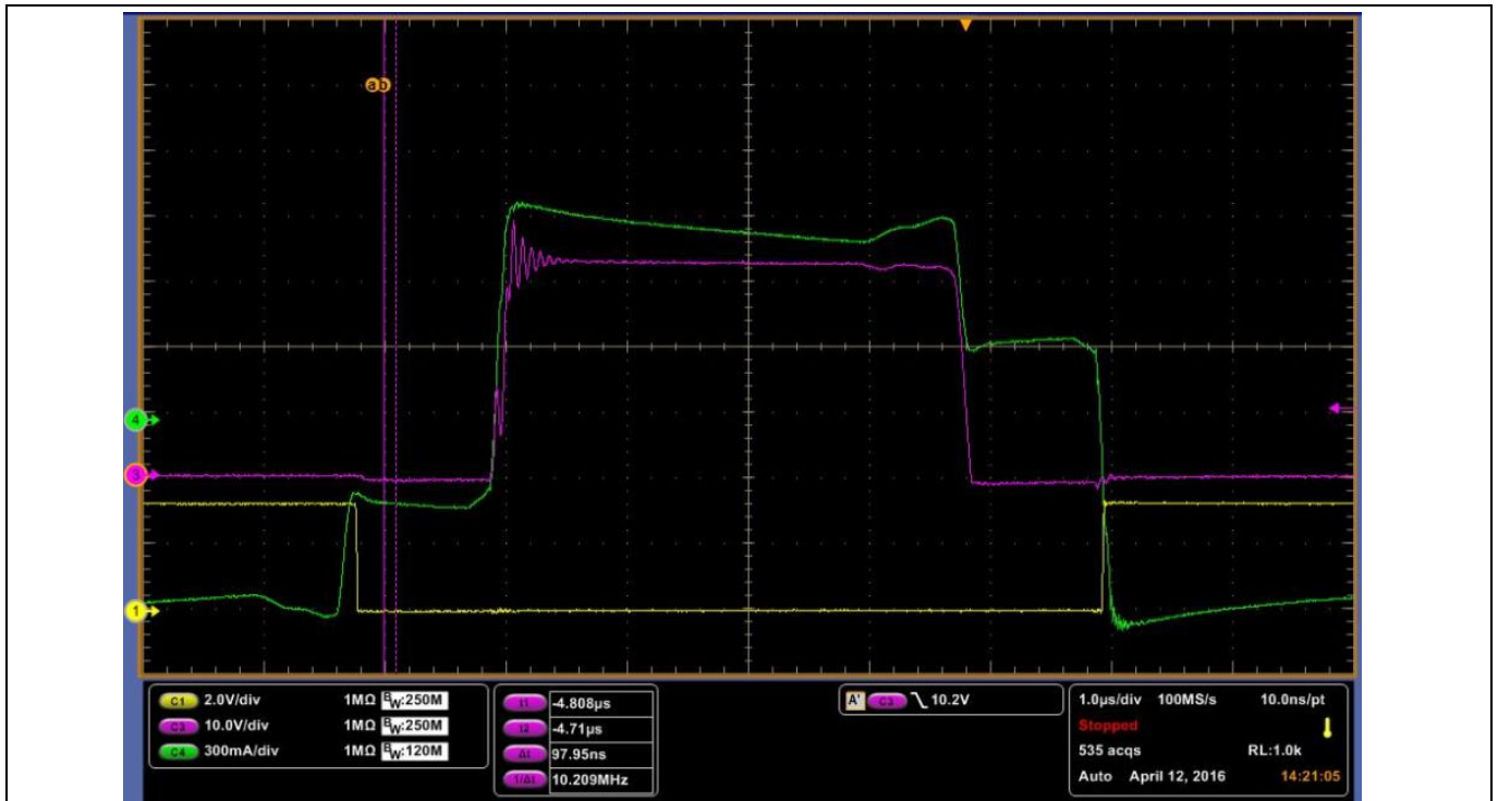
Figure 43 Synchronous MOSFET gate pulse (yellow), V_{ds} (purple) and primary current of the transformer (green)
