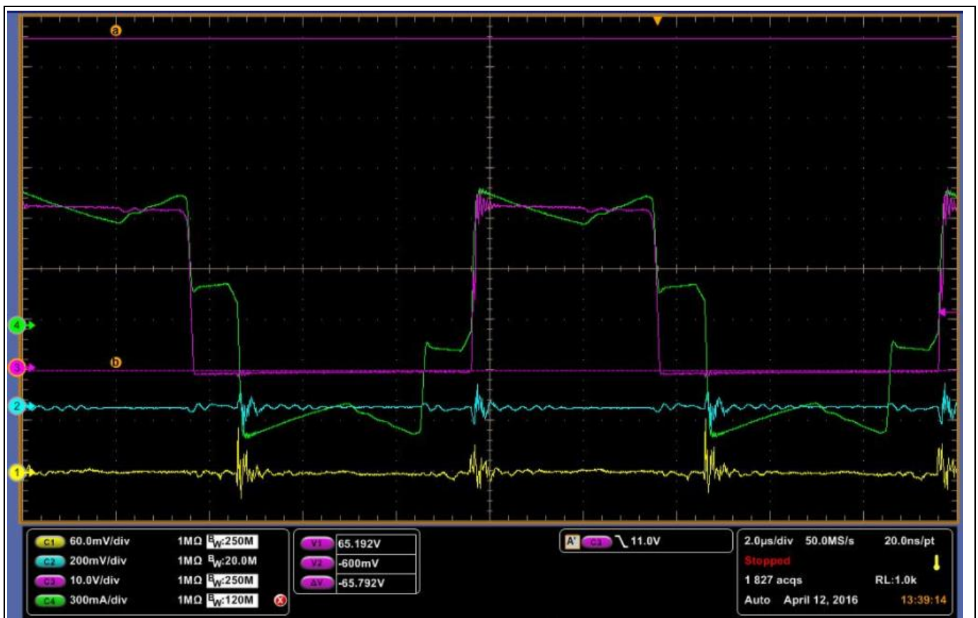
Figure 68 Synchronous mode 0 driving scheme: primary current (green), drain voltage (purple), gate voltage (yellow)
