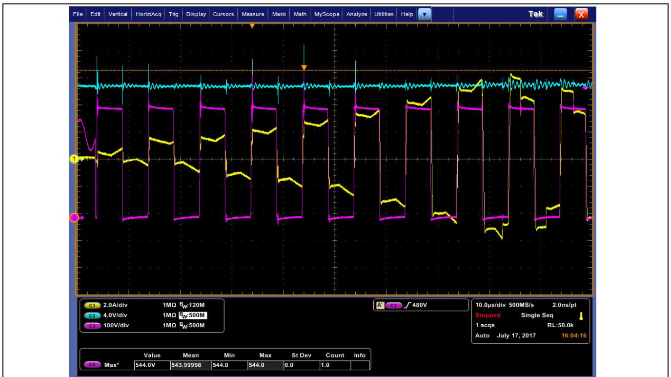
Figure 77 Short-circuit under full load at output: primary current (yellow), MOSFET_V ds (purple), output voltage (blue)
