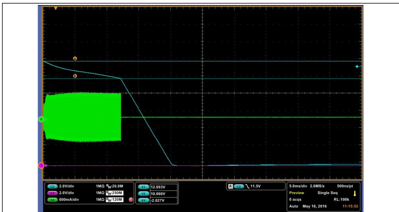
Figure 49 Cycle-by-cycle limitation in an output short-circuit event: primary current (green), output voltage (blue)
