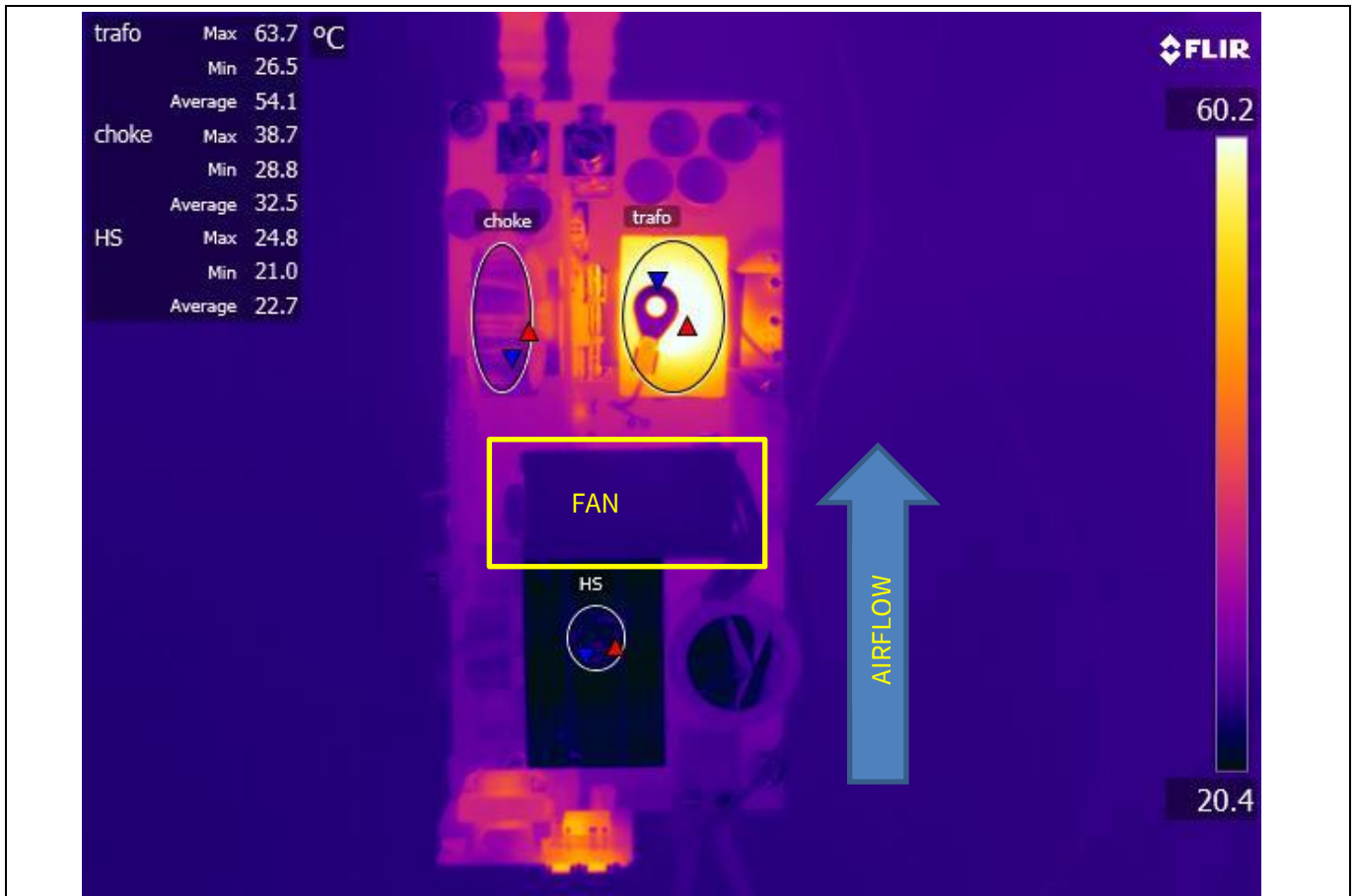
Figure 82 Board thermal map at full load (67 A) at room temperature (~25°C)
