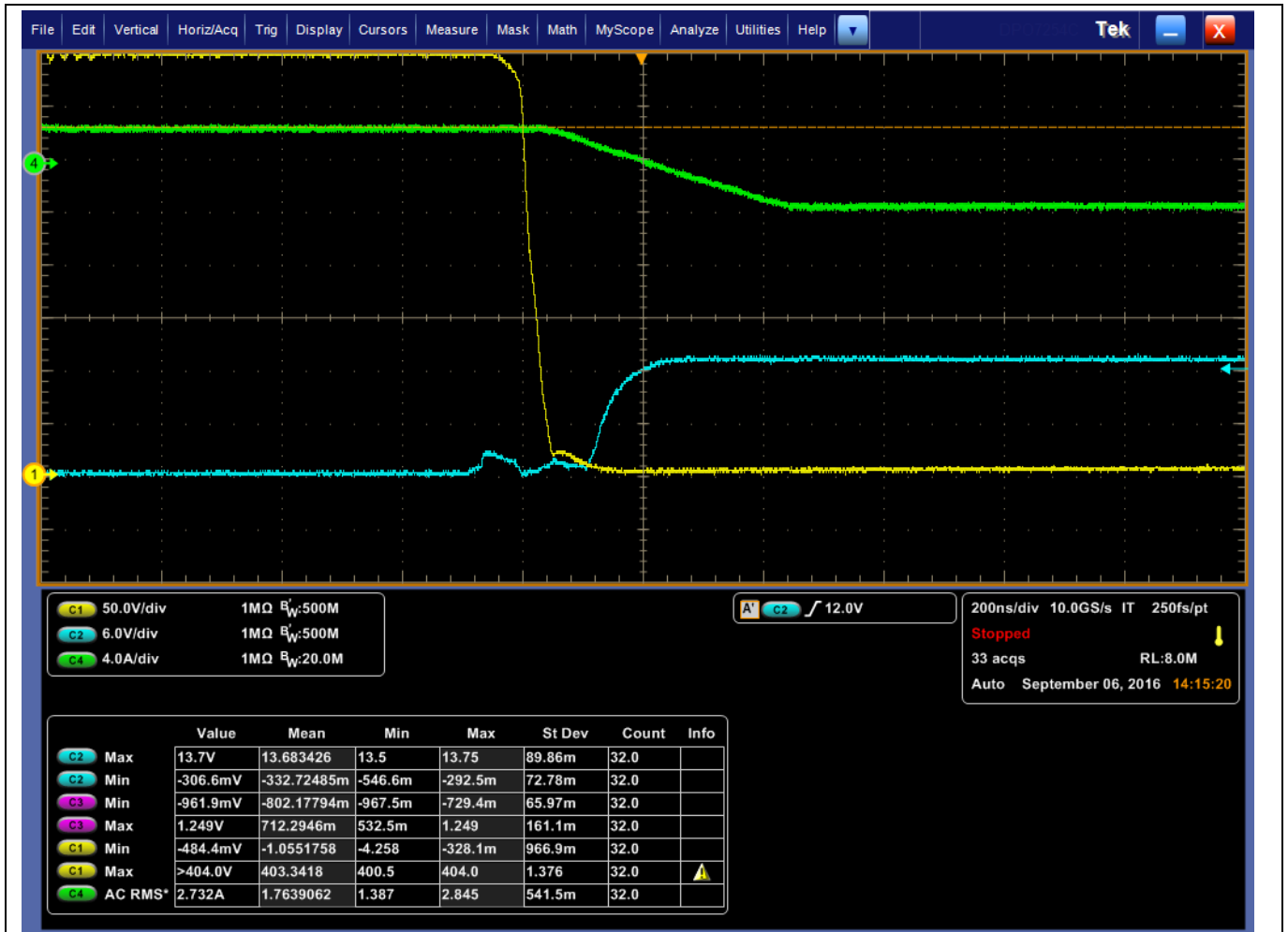
Figure 67 Leading leg achieves ZVS at 60 A. Waveforms captured on MOSFET B: primary current (green), drain voltage (yellow) and gate voltage (blue)
