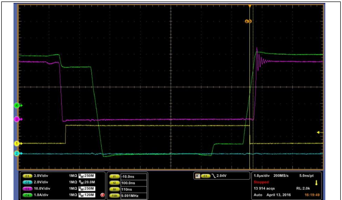
Figure 70 Synchronous mode 2 driving scheme: primary current (green), drain voltage (purple), gate voltage (yellow)
