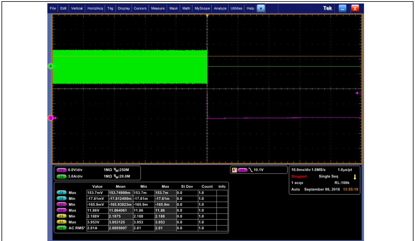
Figure 76 Short-circuit under full load at output: primary current (green), output voltage (purple)
