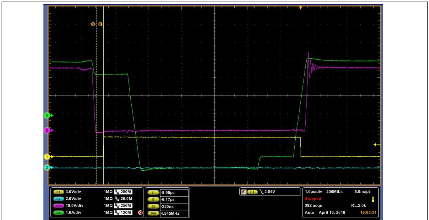
Figure 42 Synchronous MOSFET gate pulse (yellow), V_{ds} (purple) and primary current of the transformer (green)– the turn-on delay is highlighted
