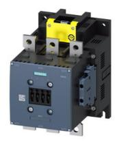
Power contactor, AC-3 225 A, 110 kW / 400 V Coil AC 50/60 Hz and DC 200-277 V x (0.8-1.1) F-PLC input 24 V DC 3-pole size S10 Auxiliary contacts 2 NO + 2 NC Main circuit: Busbar Control and auxiliary circuit: screw terminal
