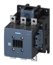
power contactor, AC-3 300 A, 160 kW / 400 V, AC (50-60 Hz) / DC operation 42-48 V AC/DC auxiliary contacts 2 NO + 2 NC 3-pole, frame size S10 busbar connections drive: conventional screw terminal
