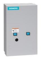
2-speed 3-phase motor starter, Size 0, Two separate windings, Constant or variable torque, Solid-state overload relays, Low Spd OLR range 0.75-3.4A, High Spd OLR range 0.75-3.4A, Enclosure NEMA type 1, Indoor general purpose use
