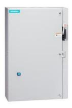
Non-reversing motor starter, Size 4, Three phase full voltage, Solid-state overload relay, OLR amp range 50-200A, 110V 50Hz / 120V 60Hz coil, Combination type, 200A non-fusible disconnect, Enclosure NEMA type 1, Indoor general purpose use, Standard width enclosure
