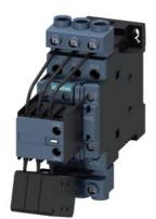
Capacitor contactor, AC-6b 33 kVAr, / 400 V 1 NO + 2 NC, 110 V DC 3-pole, Size S0 screw terminal
