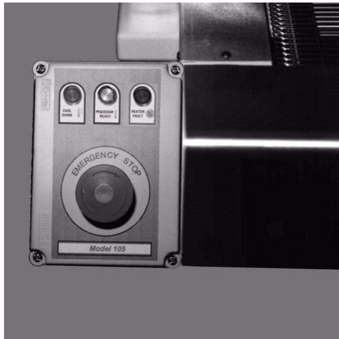
Emergency Stop Enclosure
