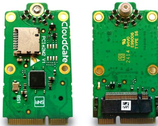
Image: Front side and back side of the M.2 to MiniPCIe adapter
