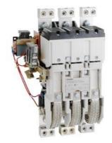
Mechanically held lighting contactor, Contactor amp rating 400A, 0 N.C. / 2 N.O. poles, 277VAC 60HZ coil, Non-combination type, Enclosure NEMA type (open), No enclosure
