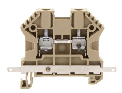
Feed-through terminal, Screw connection, Mounting type: Mounting rail TS 35/7.5, Rated cross-section: 4 mm², Width: 6 mm, Colour: Grey
