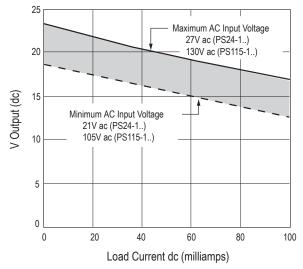
NOTE: Ripple voltage is less than 1.2V at 100 mA load
