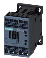
power contactor, AC-3 9 A, 4 kW / 400 V 1 NC, 12 V DC, 0.7-1.25\*US 3-pole, size S00 spring-type terminal with integrated suppressor diode spring-type terminal suitable for PLC outputs not expandable with auxiliary switch
