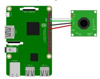
Camera 5V (black wire) to PI 3V or 5V Camera GND (black wire) to Pi Ground Camera RX (white wire) to Pi TX Camera TX (green wire) to Pi RX
