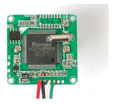
If you'd like to get NTSC video out to connect to a TV or monitor, solder another black wire to the second Ground pin, and a yellow wire to the CVBS pin.
