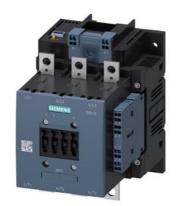
power contactor, AC-3 150 A, 75 kW / 400 V AC (50-60 Hz) / DC operation 96-127 V AC/DC auxiliary contacts 2 NO + 2 NC 3-pole, frame size S6 busbar connections drive: electronic with PLC interface 24 V DC spring-loaded terminal
