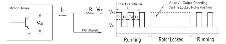
$\begin{array}{lll} \mbox{Output Type : Open Collect} & \mbox{N=R.P.M ; T= 60/N (Sec.) ; FG=1/T*2 (Hz) ; N=FG*30} \\ V_{CE} (sat)=0.5V(Max.) & V_{FG}=Maxi mum operation voltage \\ Ic=5mA (Max.) & R \geqslant V_{FG} / Ic \end{array}$
