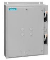
Duplex starter W/O alternator, Size 1, Three phase full voltage, Amb compensate bimetal OLrelay Contactor amp rating 27Amp 110V 50HZ / 120V 60HZ coil, Combination type, Two 30A disconnect switches, Encl NEMA type 4X 304 S-steel Water/dust tight noncorrosive
