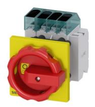
Load disconnector 3LD3, lu 25 A Main switch 3-pole + N Rated operating capacity at AC-23 A at 400V 9.0kW Front plate mounting Basic switch with Central hole mounting 22.5mm Toggle drive red / yellow 66x66 mm with auxiliary switch 1OE + 1S
