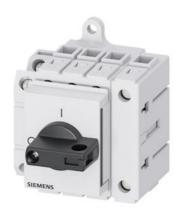
Load disconnector 3LD3, lu 40 A Main switch 3-pole + N Rated operating capacity at AC-23 A at 400 V 18.5 kW Installation in distribution boards, Basic switch with selector knob black with auxiliary switch 1OE + 1S
