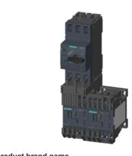
Load feeder fuseless, Reversing duty 400 V AC, Size S00 5.50...8.00 A 230 V AC Spring-type terminal for installation on standard mounting rail Type of coordination 1, Iq = 150 kA 1 NC (contactor)
