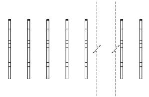
NOTE: CONTACTS ARE HELD IN A CARRIER FOR EASE OF ASSEMBLY
