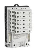
Electrically held lighting contactor, (convertible to mech. held), Amp rating 30A (tungsten 20A), 5 N.C. / 3 N.O. poles, 347V 60Hz coil, Non-combination type, Enclosure NEMA type (open), No enclosure
