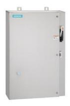
Non-reversing motor starter, Size 3, Three phase full voltage, Solid-state overload relay, OLR amp range 25-100A, 208VAC 60Hz coil, Combination type, 125A circuit breaker, Encl NEMA type 4X 304 S-Steel, Water/dust tight noncorrosive, Extra-wide enclosure
