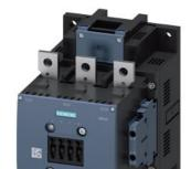
power contactor, AC-3 300 A, 160 kW / 400 V, AC (50-60 Hz) / DC operation 110-127 V AC/DC auxiliary contacts 2 NO + 2 NC 3-pole, frame size S10 busbar connections drive: conventional screw terminal NEMA version
