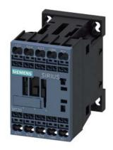
power contactor, AC-3 9 A, 4 kW / 400 V 1 NO, 24 V DC 0.7-1.25\*Us 3-pole, size S00 spring-type terminal with integrated diode, suitable for PLC outputs not expandable with auxiliary switch
