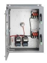
Duplex starter with alternator Size 3 Three phase full voltage Solid-state overload relay OLR amp range 25-100A 110VAC 50Hz / 120VAC 60Hz Coil Combination type Two 100A disconnect switches Encl NEMA type 4 painted steel Water/dust tight weather proof
