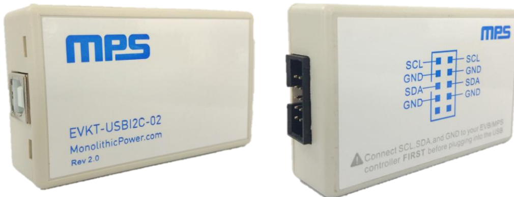
Figure 3: EVKT-USBI2C-02 Communication Interface
