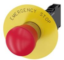
EMERGENCY STOP mushroom pushbutton, 22 mm, round, metal, shiny, red, 40 mm, positive latching, acc. to EN ISO 13850, pull-to-unlatch mechanism, with yellow backing plate, inscription: EMERGENCY STOP, with holder, 1 NO+1 NC, screw terminal, Z=20-unit packaging
