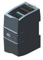
SIPLUS S7-1200 SM 1222 16DQ RLY based on 6ES7222-1HH32-0XB0 with conformal coating, -40...+70 °C, start up -25 °C, digital output 16 DQ, relay 2 A
