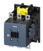
Power contactor, AC-3 265 A, 132 kW / 400 V Coil AC 50/60 Hz and DC 200-277 V x (0.8-1.1) F-PLC input 24 V DC 3-pole size S10 Auxiliary contacts 2 NO + 2 NC Main circuit: Busbar Control and auxiliary circuit: screw terminal
