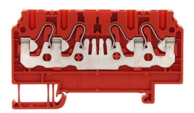
Feed-through terminal, Push-in connection, Mounting type: Mounting rail TS 35/7.5, Rated cross-section: 1.5 mm², Width: 4.1 mm, Colour: Red
