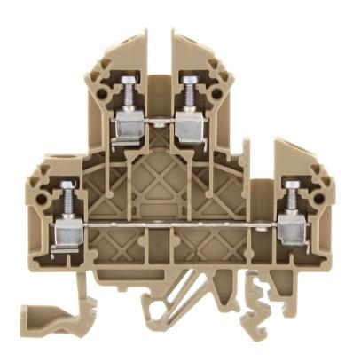
Ex double-level terminal ATEX-certified, Screw connection, Mounting type:Mounting rail TS 35/7.5 and TS 32, Rated cross-section: 2.5 mm², Width: 5 mm, Colour: Beige
