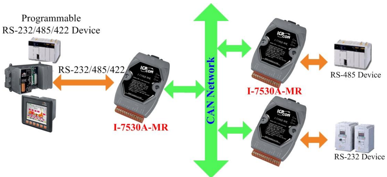
Figure 1-1: The application architecture in the Pair Connection mode.
