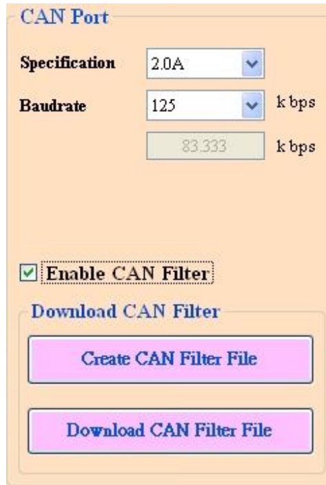
Figure 3-11: The CAN port of I-7530A-MR configuration.
