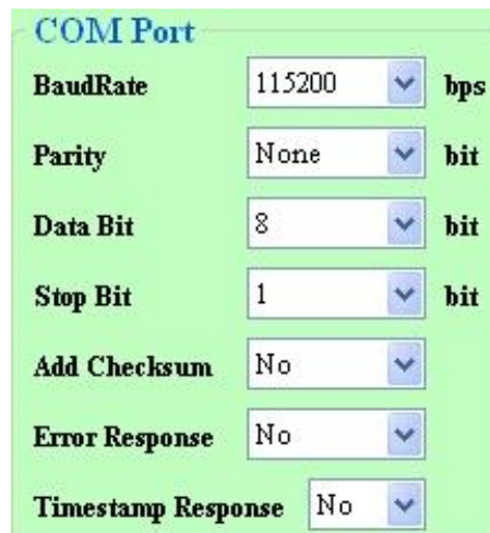
Figure 3-10: The COM port of I-7530A-MR configuration.
