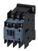
power contactor, AC-3 9 A, 4 kW / 400 V 1 NO + 1 NC, 220 V AC, 50 Hz 240 V, 60 Hz, 3-pole Size S0 ring cable lug connection
