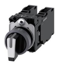
Selector switch, illuminable, 22 mm, round, plastic with metal front ring, white, selector switch, short, 3 switch positions I>O<II, momentary contact type, actuating angle 2x45°, 10:30h/12h/13:30h, with holder, 1 NO+1 NC, 1 NO+1 NC, screw terminal, Z=20-unit packaging
