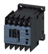
Power contactor, AC-3 7 A, 3 kW / 400 V 1 NO, 400 V AC, 50 Hz 400-440 V, 60 Hz, 3-pole, Size S00, ring cable lug connection
