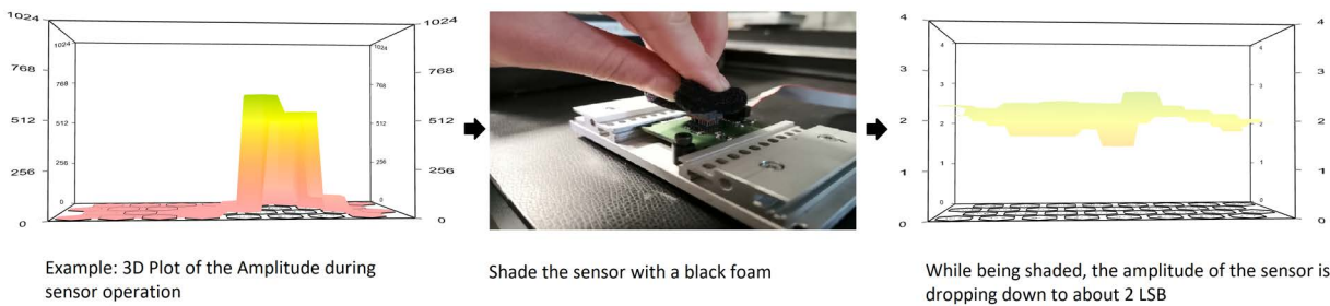
Figure 39: Blinding Sensor for Xtalk Calibration
