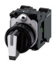
Selector switch, illuminable, 22 mm, round, plastic, white, selector switch, short, 3 switch positions I-O-II, latching, 10:30h/12h/13:30h, with holder, 1 NO, 1 NO, spring-type terminal, with laser labeling, upper case
