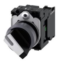
Selector switch, illuminable, 22 mm, round, plastic with metal front ring, white, selector switch, short, 2 switch positions O-I, latching, actuating angle 90°, 10:30h/13:30h, with holder, 1 NO, screw terminal, with laser labeling, upper case
