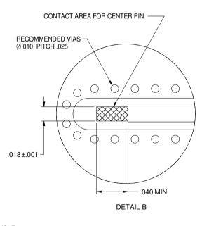
RECOMMENDED PCB LAYOUT NOTE: THIS PATTERN IS FOR REFERENCE ONLY. PATTERN MAY VARY DEPENDING ON BOARD TYPE, SPECIFIC ELECTRICAL OR MECHANICAL REQUIREMENTS.
