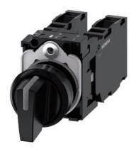
Selector switch, Illuminable 22 mm, round, plastic, black, knob, short 3 switch positions I-O-II, latching, 10:30h/12h/13:30h, with holder, 1 NO, 1 NO, screw terminal
