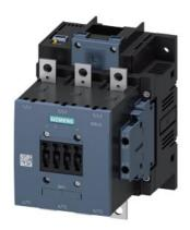
power contactor, AC-3 150 A, 75 kW / 400 V AC (50-60 Hz) / DC operation 21-27 AC/DC, 3 V auxiliary contacts 2 NO + 2 NC 3-pole, frame size S6 busbar connections drive: electronic with PLC interface 24 V DC screw
