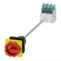
SENTRON, Switch disconnector 3LD, emergency switching-off switch, 3-pole, lu: 25 A, operating power / at AC-23 A 400 V: 9.5 kW, floor mounting with door coupling, rotary operating mechanism, Red / yellow, central mounting 22.5 mm of the handle
