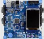
The Keil MCB1760 Evaluation Board introduces the new NXP LPC1760 family of ARM Cortex-M3 processor-based devices, allowing you to create and test working programs for this advanced architecture. The MCB1760 has a wide range of interfaces making it a great starting point for your next Cortex-M3 project.
