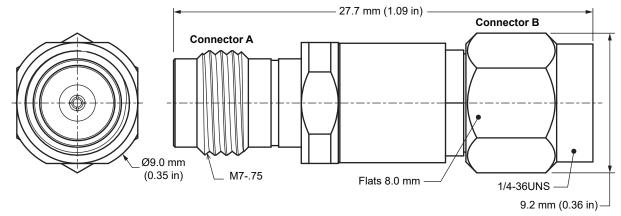
Figure 1. Product Dimensions for the ADP-2.4F-2.92M Adapter
