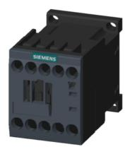
Power contactor, AC-3 7 A, 3 kW / 400 V 1 NC, 480 V AC, 60 Hz 3-pole, Size S00 screw terminal
