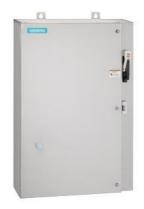
Non-reversing motor starter, Size 3, Three phase full voltage, Solid-state overload relay, OLR amp range 25-100A, Combination type, 100A non-fusible disconnect, Encl NEMA type 4X 304 S-Steel, Water/dust tight noncorrosive, Extra-wide enclosure
