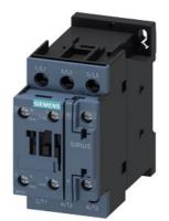
power contactor, AC-3 9 A, 4 kW / 400 V 1 NO + 1 NC, 220 V AC 50 / 60 Hz, 3-pole, Size S0, screw terminal
