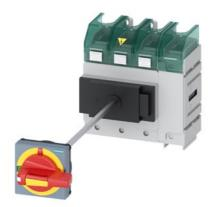
SENTRON, Molded case switch 3LD5 UL, Emergency switching-off, 4-pole, certified according to UL489 UL60947-4-1 and IEC60947-3, UL: 150A, SCCR 50kA at 480VAC, Operating power at 480VAC 3-phase: 100hp, IEC: 160A, Operating power at AC-23A at 400V: 75kW, floor mounting with door coupling rotary operating mechanism, defeatable, emergency switching-off, 4-hole mounting of the handle, without tolerance compensation, incl. terminal covers for the infeed side
