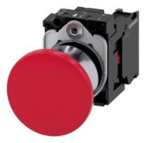
Mushroom pushbutton, 22 mm, round, metal, shiny, red, 40mm, latching, pull-to-unlatch mechanism, with holder, 1 NC, screw terminal, with laser labeling, lower case
